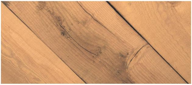
Band sawn texture from inside the antique beams.
